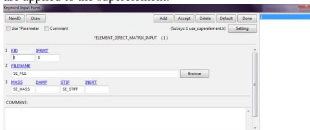
Figure 1.2 Control Card for represent the superelement results in the reduced FE mode
